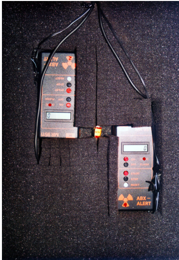
Fig. 4: Radioactive source (uranium oxide) with two 180° shifted Geiger-Müller counters
